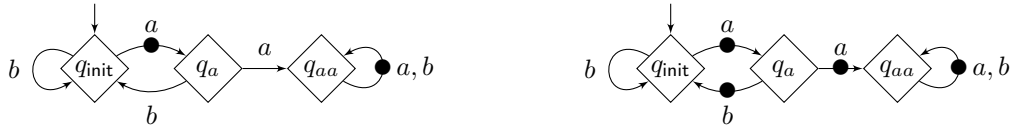
Figure 1: A DBA (left) and its unique saturation (right). Transitions labeled with a \bullet symbol are the Büchi transitions. In figures, automaton states are depicted with diamonds.
